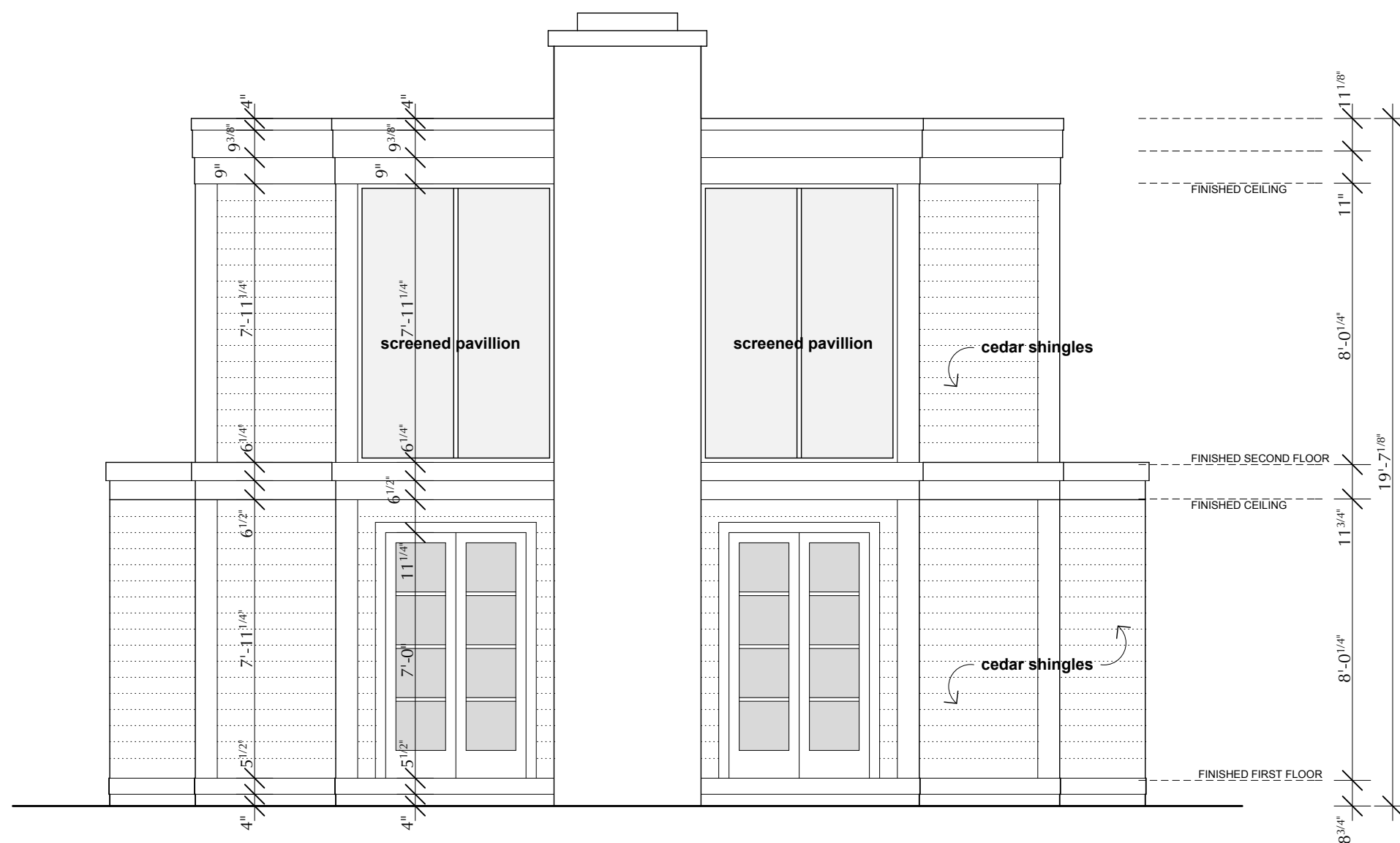
3 A2 NORTH ELEVATION SCALE = 1/4" = 1'-0"
