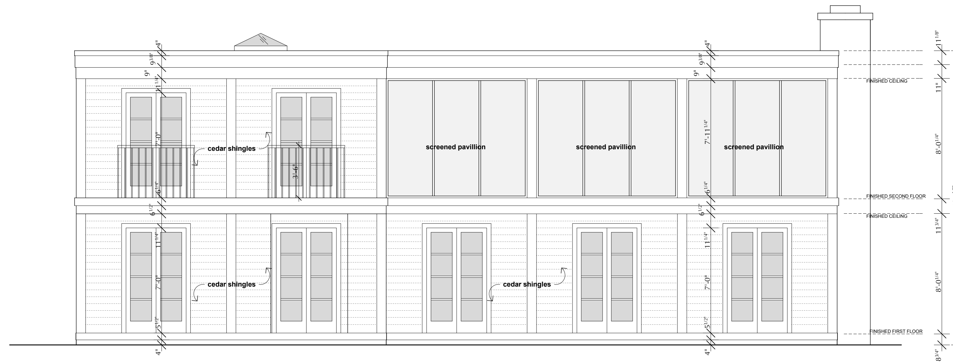
2 A2 EAST ELEVATION SCALE = 1/4" = 1'-0"
